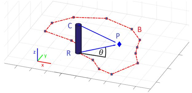
Fig. 4: Illustration of the underlying geometry for determining the keep off area. The current robot's position  $R$  and its camera position  $C$  are depicted as a blue cylinder.  $B$  denotes the virtual border polygon and  $P$  the last known marker position.
