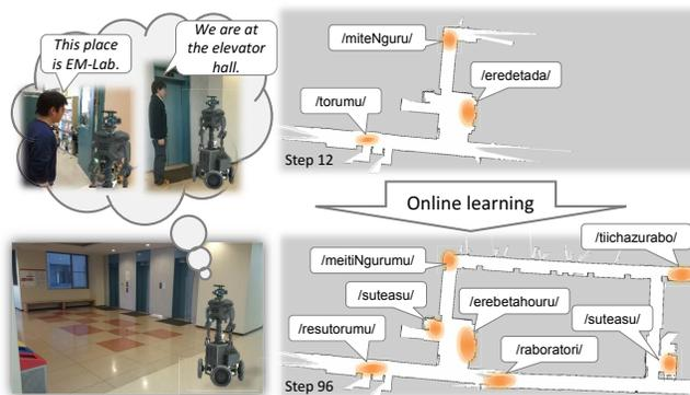
Fig. 1. Overview of online learning of spatial concepts and an environmental map; We aim to develop a method that enables mobile robots to learn spatial concepts, a lexicon and an environmental map sequentially from interaction with an environment and human, even in an unknown environment without prior knowledge.
