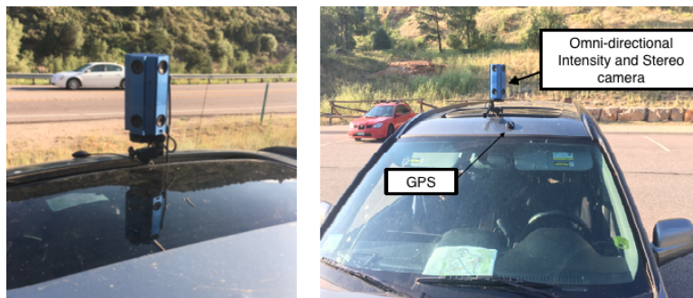
Fig. 1 Camera and GPS setup. Camera settings (e.g. exposure level) were optimized at the start of each run in order to get the best intensity and stereo image.
