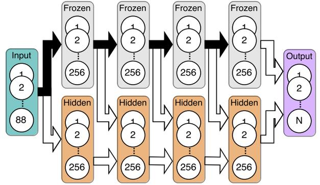
Figure 2: *Progressive Neural Network (ProgNet) used in our experiments. The arrows represent dense connections between each layer. The black arrows show frozen weights from the transferred representations. The number of outputs ( $N$ ) varies depending on the experiment.*
