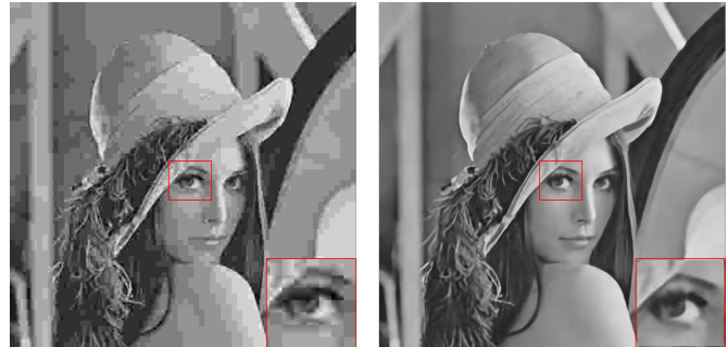
Fig. 1. Left: the JPEG-coded image (PSNR = 27.33 dB) with QF = 5, where we could see blocking artifacts, ring effects and blurring on the eyes, abrupt intensity changes on the face. Right: the decoded image (PSNR = 31.14 dB) by our proposed compression framework at the same bit rate with left, where the compression artifacts vanished and generate more details.
