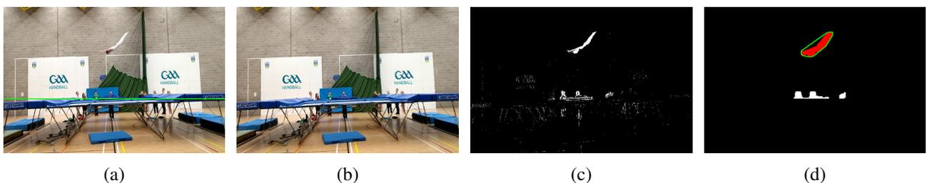
Figure 3: Processed images. (a) Original frame. (b) Background model. (c) Foreground mask. (d) Body silhouette and convex hull after erosion and dilation.
