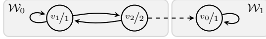
Fig. 7. Additional memory allows Player 0 to remain in v_1 longer and longer, thus decreasing the potential for disturbances.
