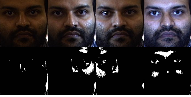
Fig. 3. Specular highlight detection results on images under various lighting conditions. Top row: original images; bottom row: detected highlight masks.
