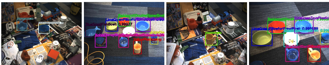
Figure 13. Objects with similar shapes and colors detected in challenging environments. The detector was trained on synthetic images only.
