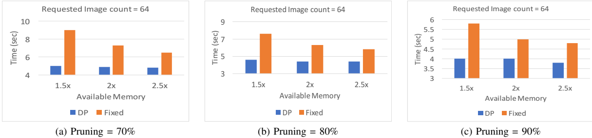
Fig. 6: Fixed batch size (baseline) time vs Time outputted from Dynamic Programming for AlexNet with 70%, 80% and 90% pruning.
