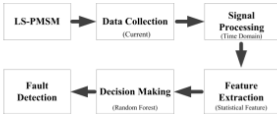
Fig. 4. The flowchart diagram of fault diagnosis system.
