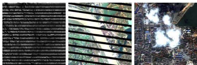
(a) Dead lines in Aqua MODIS band 6 (b) Landsat ETM+ SLC-off (c) QuickBird image with thick cloud cover
