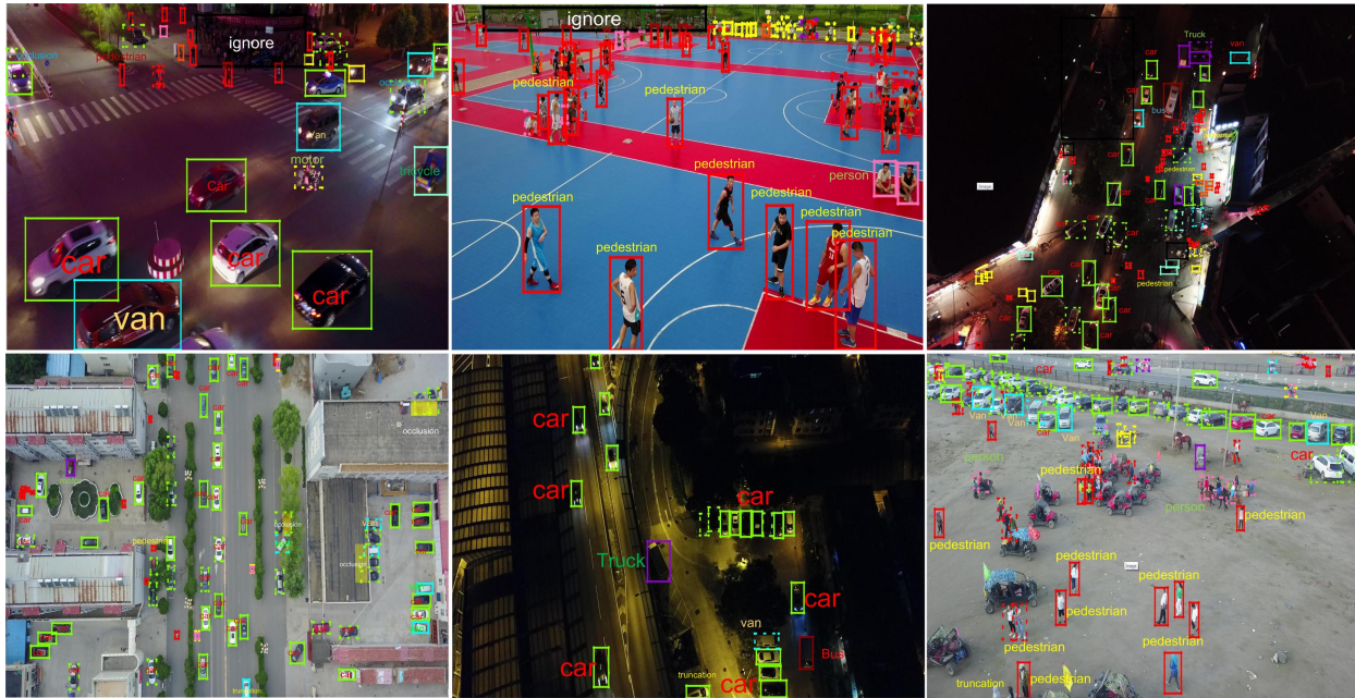
Fig. 3: Some annotated example images of (Task 1) object detection in images. The dashed bounding box indicates the object is occluded. Different bounding box colors indicate different classes of objects. For better visualization, we only display some attributes.
