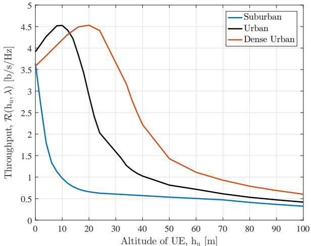
Fig. 4. In an urban area achievable throughput (channel capacity) of an omnidirectional UAV at altitude of 100 m is only 12% of a ground user and 10% of its maximum at the optimum altitude, *i.e.*  $h_u = 10$  m. In this case feasible operational range of UAV altitude is very limited.
