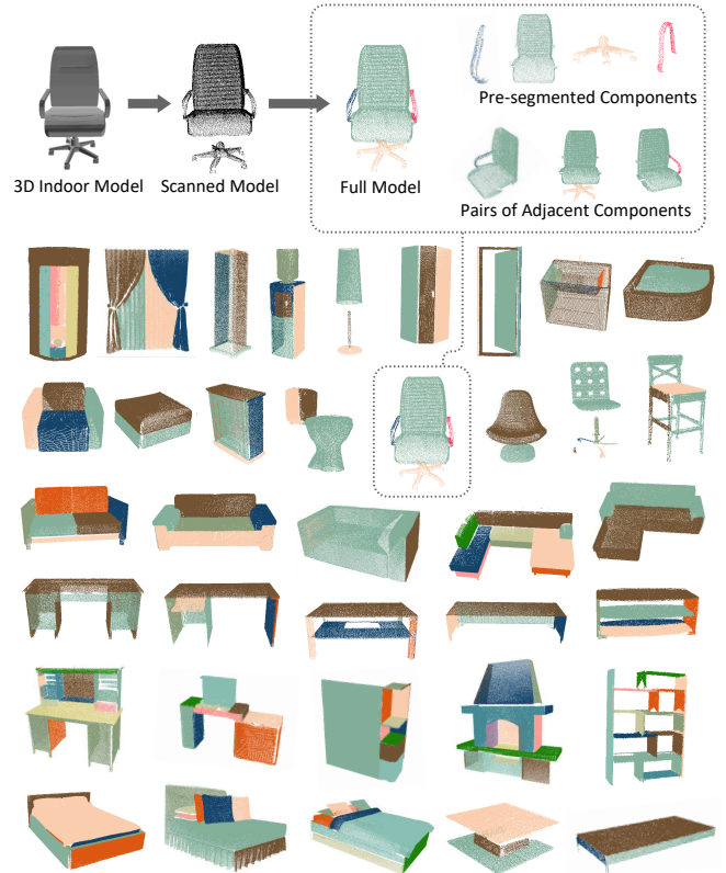
Fig. 4. The database \mathcal{M} of 3D indoor models. For each model, such as the chair, we virtually scan it and put it into \mathcal{M} . Then, we segment it into pre-segmented components and put them into \mathcal{M} . We also put the pairs of adjacent pre-segmented components into \mathcal{M} .
