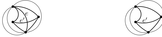
(a) Empty kite with crossing edges e and e' . The original edge e got parallel dummy edges during the execution of the augmentation step. (b) After the removal of the original edge e , the empty kite becomes a divided quadrangle containing e' as inner edge.
