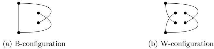
Fig. 15: Embedded graph configurations of 1-plane graphs that cannot be drawn with straight-line edges.
