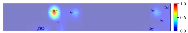
Figure 5: Heat map visualization of the relative importance of each pixel in the visual input of an agent towards the velocity command. Red regions have the most influence on the control command, whereas blue regions contribute the least.
