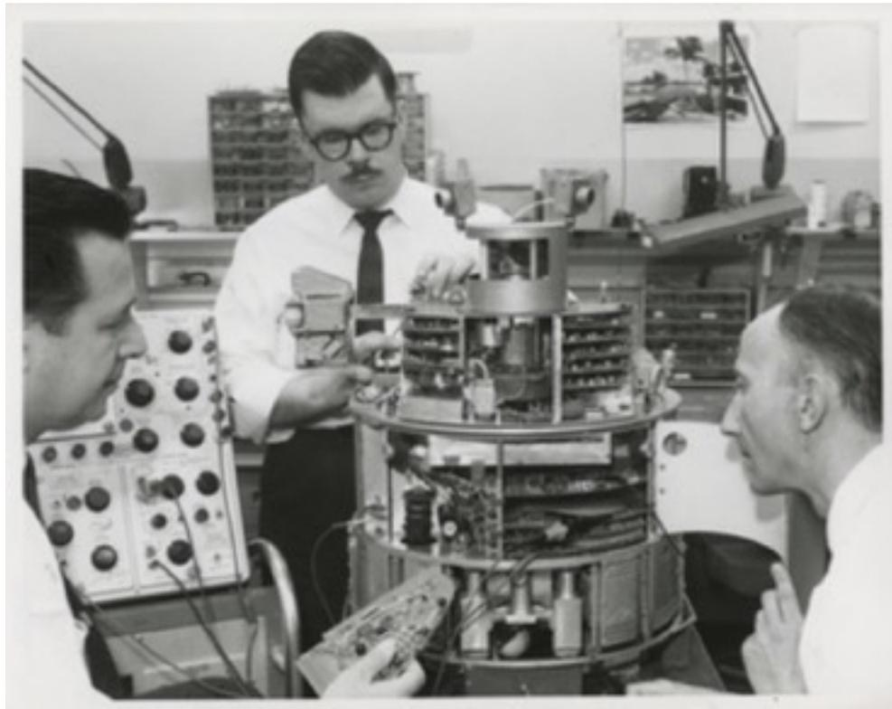
Figure 1.2: "Mar 31 1965" Photo No. 73738; UNDER THE SKIN.... Leonard Scheer, left, William Whitmore with automaton, and Dennis Walters have removed the bumper and cover from automaton to examine the complex electronics.". Photo of three men examining and working on the electronics of a robot in a laboratory/shop environment. (Source: [cyberneticzoo.com](http://cyberneticzoo.com))
