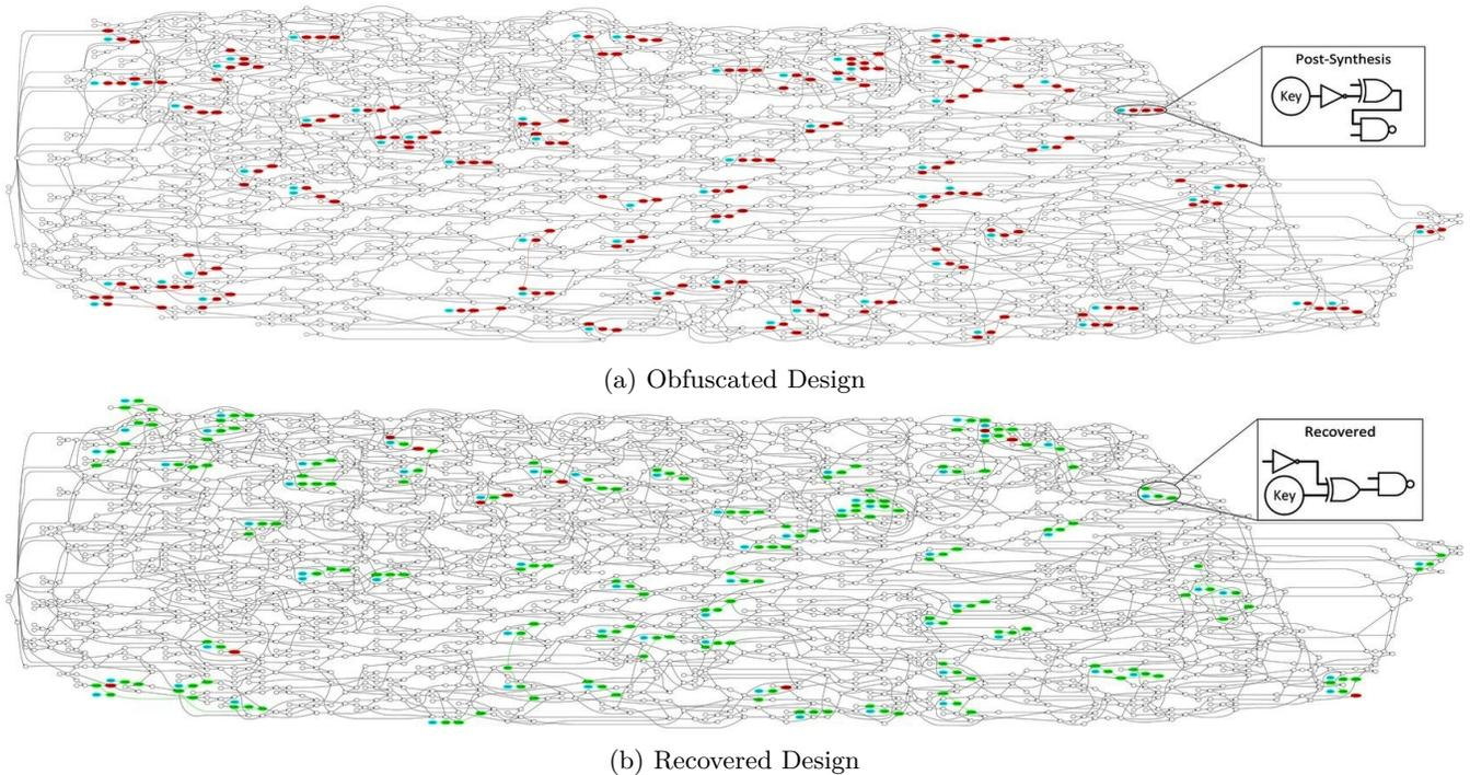
Fig. 6: Visual representation of SAIL recovery on C6288, with 95% accuracy. Each node is a gate and edges are connections. Green nodes are correctly recovered, and red nodes are incorrectly recovered. Cyan nodes are key inputs.
