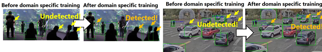
Figure 1: Object detection results of the test image, before and after domain specific training.
