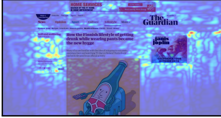
Figure 9: Activation Maps of our Ad Detection Model. The most salient features appear to be the surroundings of ads rather than their visual content.
