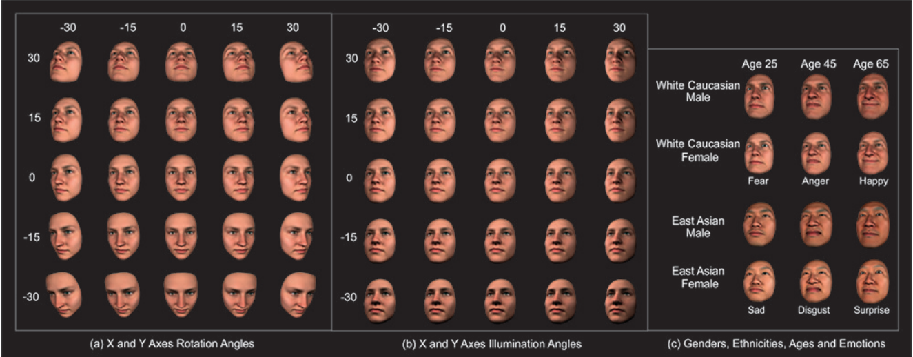
Figure 1. Extrinsic (a and b) and Intrinsic (c) Factors of Variance of the Generative Model of 3D Faces. We generated 2,000 different identities and used the extrinsic and intrinsic factors of face variance to combinatorially generate 26M face images.
