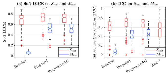
Fig. 5: Results of shadow confidence estimation. (a) Soft DICE of the baseline, the proposed method and the proposed method with attention gates (proposed+AG) on  $S_{test}$  and  $M_{test}$ . (b) Interclass correlation (ICC) of the baseline, the proposed method and the proposed+AG on  $S_{test}$  and  $M_{test}$ . Additionally, ICC of the human performance is shown as Anno\* for  $S_{test}$ .
