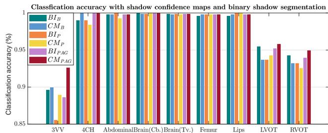
Fig. 8: Comparison of classification accuracy between using shadow confidence maps and using shadow segmentation.  $BI_B$ ,  $BI_P$  and  $BI_{P+AG}$  are networks with binary shadow segmentation from the baseline, the proposed method and the proposed+AG method.  $CM_B$ ,  $CM_P$  and  $CM_{P+AG}$  are the same networks as in Tabel IV.
