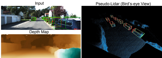
Figure 5: Pseudo-LiDAR signal from visual depth estimation. Top-left: a KITTI street scene with super-imposed bounding boxes around cars obtained with LiDAR (red) and pseudo-LiDAR (green). Bottom-left: estimated disparity map. Right: pseudo-LiDAR (blue) vs. LiDAR (yellow) — the pseudo-LiDAR points align remarkably well with the LiDAR ones. Best viewed in color (zoom in for details).
