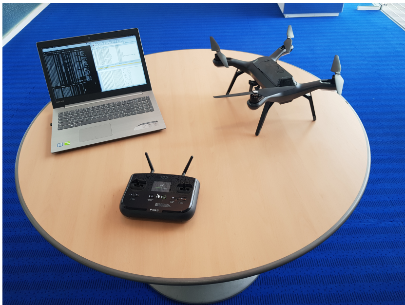
Figure 2: Our measurement set-up: the drone, the remote controller, and the laptop we used to eavesdrop the radio spectrum.
