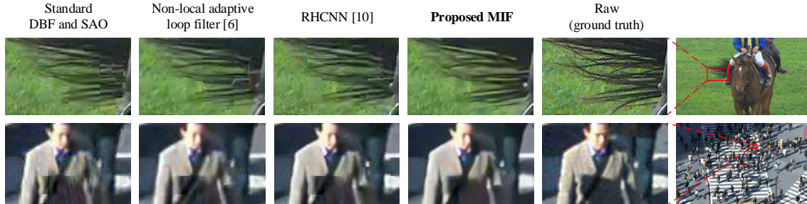
Figure 4: Comparison of subjective visual quality on sequences RaceHorses (Class C) and PeopleOnStreet (Class A) at QP = 37 .
