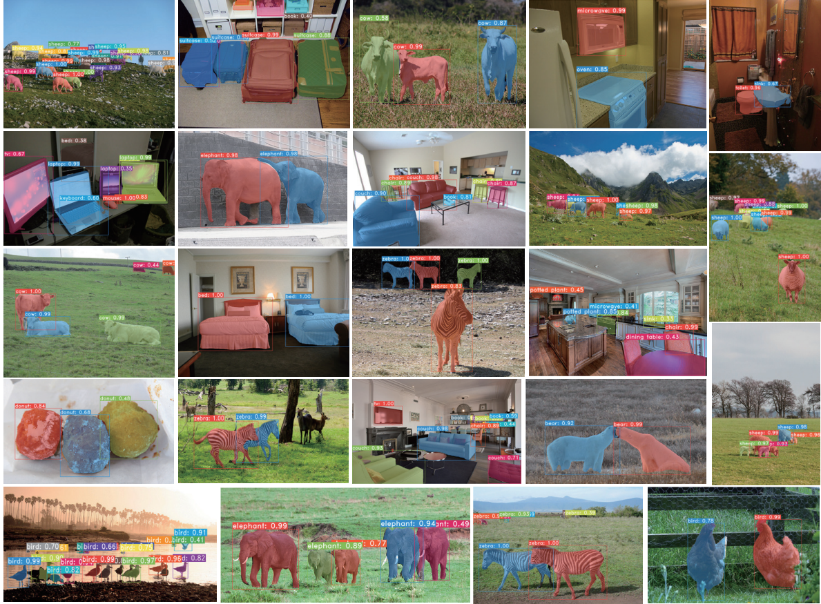
Figure 8: More YOLACT evaluation results on COCO’s test-dev set with the same parameters as before. To further support that YOLACT implicitly localizes instances, we select examples with adjacent instances of the same class.
