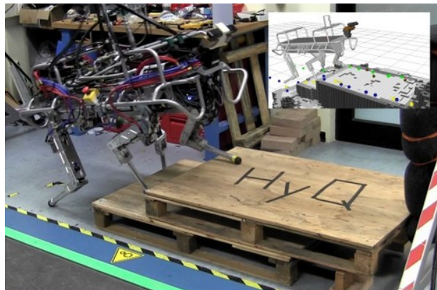
Fig. 1. The hydraulically actuated and fully torque controlled quadruped robot HyQ [2]. The inset plot shows the on-line built environment perception alongside with the planned footholds and the current on-board robot state estimate.
