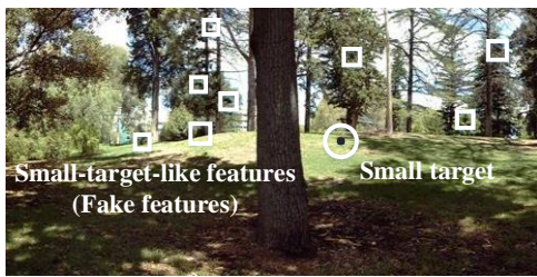
Fig. 1. A small target is moving in the cluttered natural background which contains a number of small-target-like features (or called fake features). The small target and fake features all appear as small dim speckles whose sizes vary from one pixel to a few pixels, since they are far away from the animal/camera.
