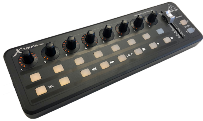
Figure 5: We used the X-Touch Mini to control an additive synthesis instrument along with a 9D MDRNN model ( dt, \text{knobs 1-8} ).
