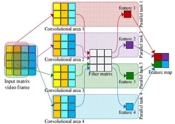
Fig. 5. Example of the parallel convolutional operation.
