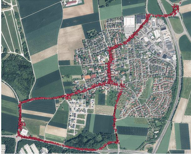
Fig. 4. Overview of the landmark-based map with landmarks depicted as red circles (●). The route in Ulm-Lehr (Germany) is about 5km long and the resulting map is comprised of 3860 landmarks.
