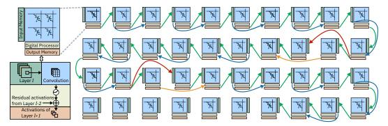
Figure 8: Mapping of ResNet-32 on a 4-by-10 array of CM cores. Each layer is mapped onto one core. Arrows indicate the communication of data between cores. Green arrows denote the propagation of activations to the adjacent layer. Blue arrows represent data movement arising from residual connections. Orange arrows indicate re-sampled residual connections, and red arrows represent communication to residual re-sampling layers.
