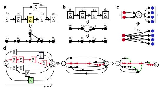
Figure 1: Illustration of representation rules. Yellow layer in **a.** represents a layer with stride = 2; green layer in **d.** represents a layers to which  $3 \times 3$  max pooling is previously applied.
