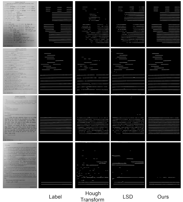
Fig. 5. Some examples of AAU segmentation. Here, the max gap of lines in Hough Transform is set to 5 and the minimum length of lines in LSD in set to 40.
