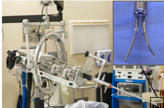
Fig. 16. This robot for transurethral HoLEP consists of a hand-held user interface and concentric tube manipulators that are actuated by an electromechanical actuation unit. Reproduced with permission.<sup>141</sup>
