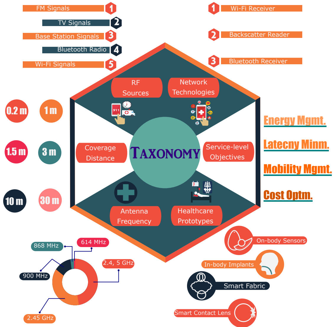
Fig. 2: Taxonomy of different features including network technologies, RF source, service-level objectives, antenna frequency, coverage distance, prototypes for backscatter communications in healthcare. The network technologies for backscatter readers/ tags include Wi-Fi receivers and Bluetooth radios. Mobility considerations for fulfilling service-level objectives consider walking (i.e., 1.1 m/s) and running (i.e., 2.2 m/s) scenarios. While most of the backscatter applications are focused on conventional transmission of the sensed data to a gateway.
