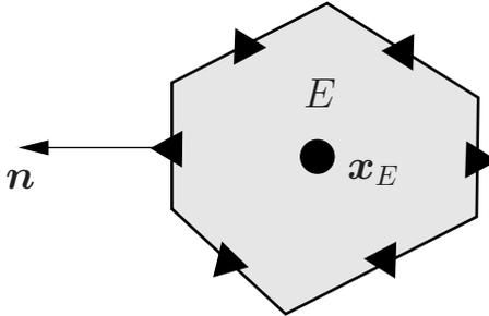
Figure 3: Schematic representation of a nodal integration cell. The integration node and its associated nodal cell is denoted by  $E$ , and the area of the nodal cell by  $|E|$ . The coordinates of the integration node are  $\mathbf{x}_E$  and the unit outward normal to the nodal cell's boundary is  $\mathbf{n}$ . The  $\blacktriangle$  stands for the 1-point Gauss rule over an edge of the nodal cell.
