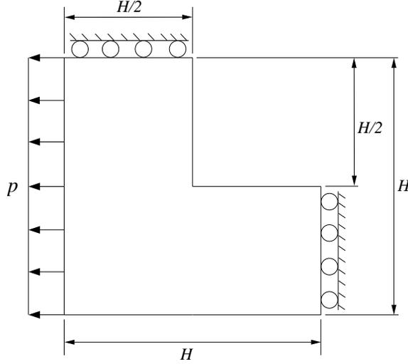
Figure 15:  $L$ -shaped domain under traction load.
