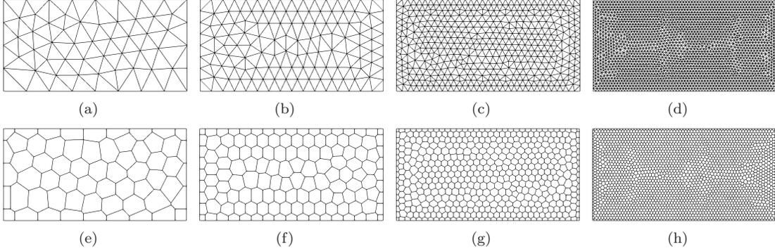
Figure 10: Sequence of background integration meshes used for the cantilever beam problem. (a)-(d) Meshes for the MEM method and (e)-(h) meshes for the NIVED method.
