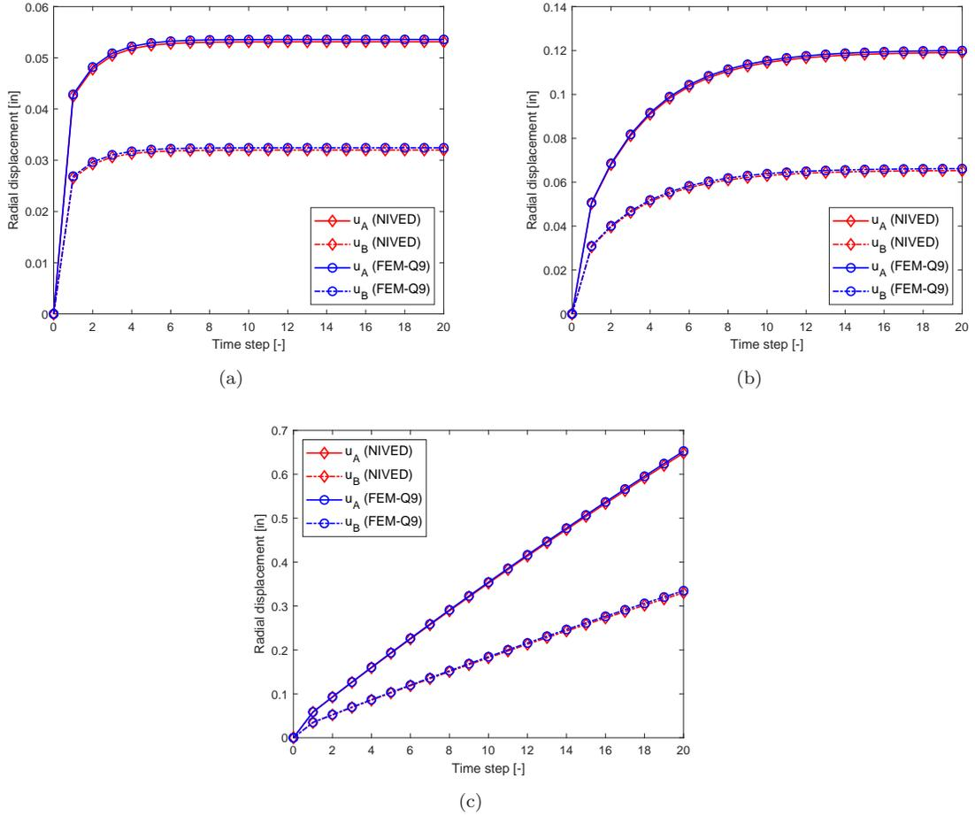
Figure 25: Thick-walled viscoelastic cylinder subjected to internal pressure. Time history of the radial displacement measured at control points  $A$  (upper curves) and  $B$  (lower curves) for three sets of viscoelastic parameters: (a)  $(\mu_0, \mu_1) = (0.7, 0.3)$ , (b)  $(\mu_0, \mu_1) = (0.3, 0.7)$  and (c)  $(\mu_0, \mu_1) = (0.01, 0.99)$ .
