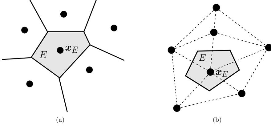
Figure 1: Construction of a nodal representative domain (shaded area) using (a) a Voronoi diagram and (b) a triangular mesh. The node and its representative cell are denoted by  $E$  and  $\mathbf{x}_E$  are the nodal coordinates.
