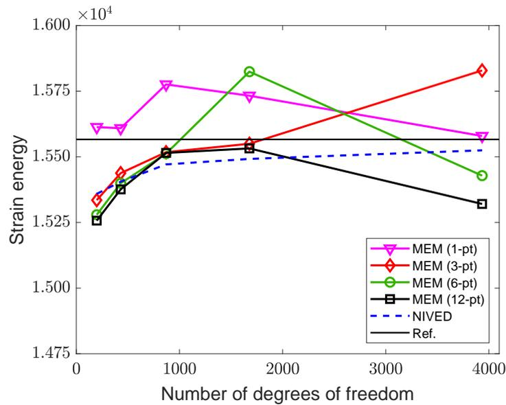
Figure 17: Convergence of the strain energy for the  $L$ -shaped domain problem. The MEM method does not uniformly approach the reference value of the strain energy, whereas the proposed NIVED scheme does.
