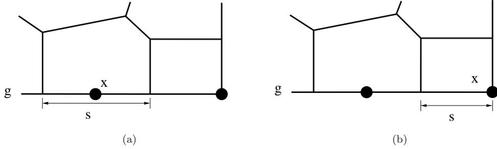
Figure 2: Schematic representation of a node located on  $\Gamma_t$  with coordinate  $\mathbf{x}_S$  and associated length of influence  $|S|$ . (a) A node located inside a boundary edge and (b) a node located at a boundary corner.
