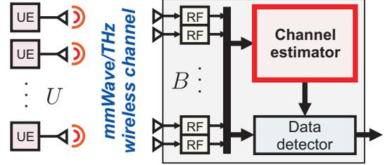
Fig. 1. Massive MU-MIMO mmWave uplink system:  $U$  UEs transmit pilots over a mmWave/THz wireless channel, which are used to estimate the channel vectors associated to each UE at the  $B$ -antenna base station.
