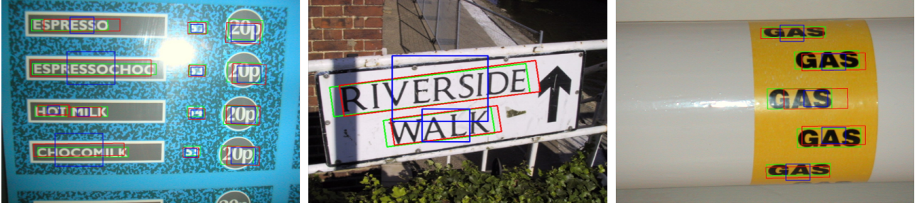
Figure 3. The view of different boxes. The blue, red and green boxes represent original anchor, learned anchor and final output box respectively. It is worth noting that the learned anchor (red) shares the same central point with the original one (blue). Viewing digitally with zooming is recommended.
