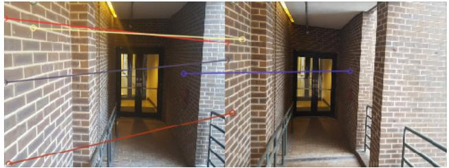
Fig. 3: An example of matched keypoint inliers after performing RANSAC. Clearly these keypoints are not abundant enough for use in pose estimation, but they serve as a good geometric check for loop closure detection.
