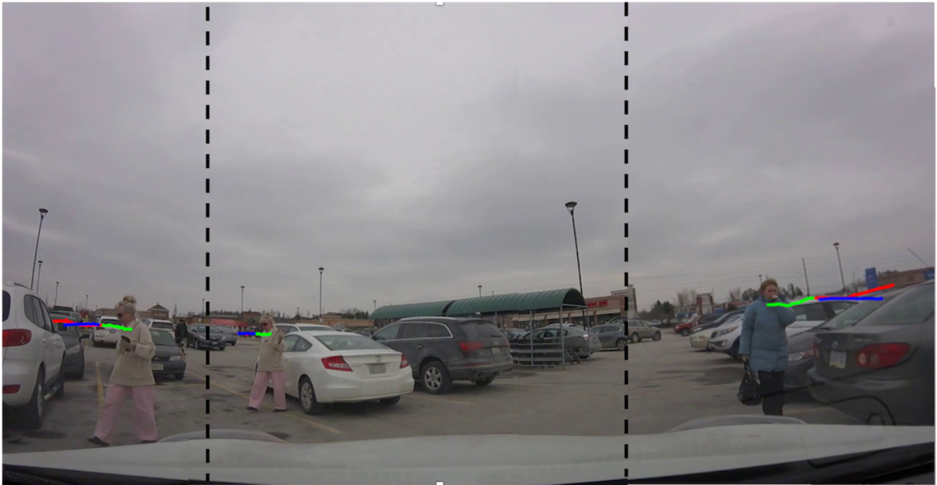
Figure 9: Visualization as a collage for three different trajectory prediction instances (in the same video). Green denotes the input to the network, Blue is the prediction and red is the ground truth. The trajectories are also a bit distorted from typical walking behaviour because of the car's (camera's) motion itself.
