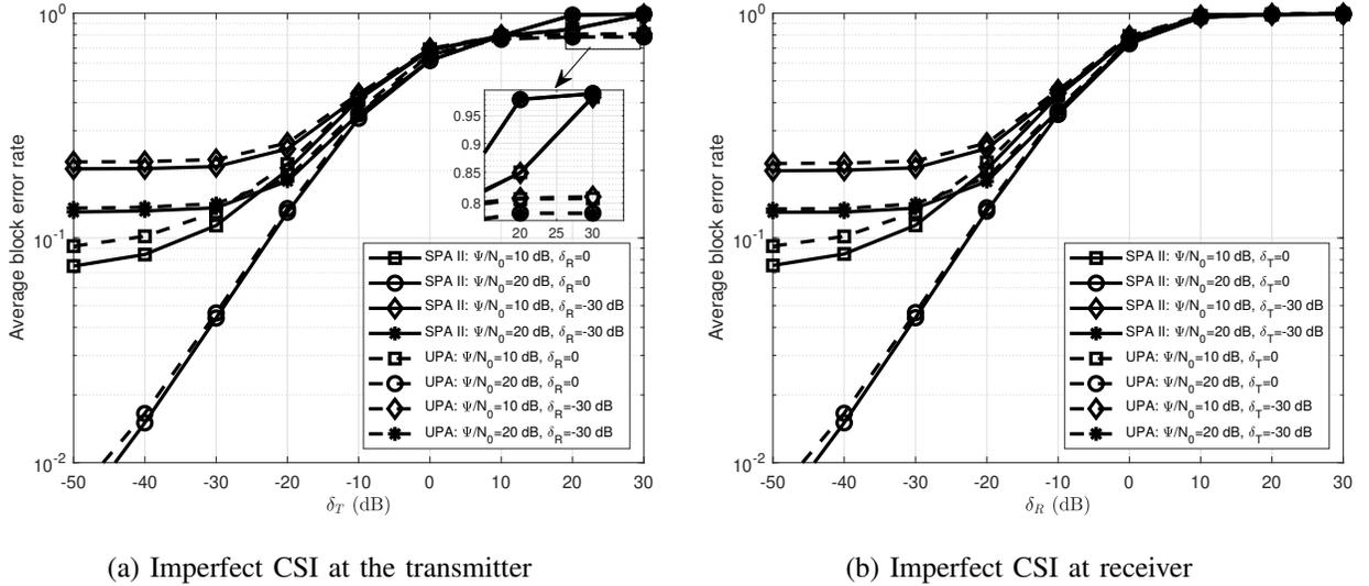
Fig. 9: Average BLER vs. the variance of channel estimation errors for imperfect CSI at the transmitter and receiver.
