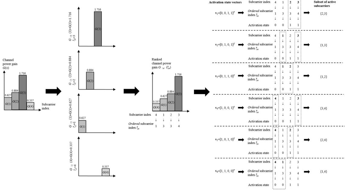
Fig. 2: SAP ordering procedure of the given example by the lexicographic ordering principle.
