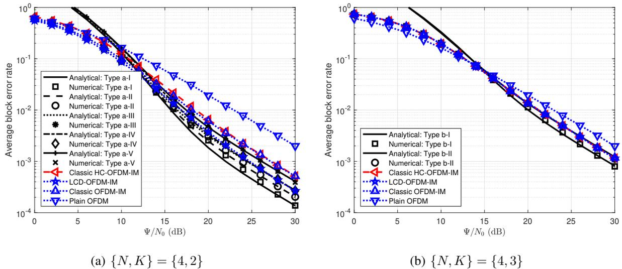
Fig. 6: Average BLER vs.  $\Psi/N_0$  with different tree architectures and different numbers of active subcarriers  $K$ , given  $N = 4$  and  $M = 2$ .
