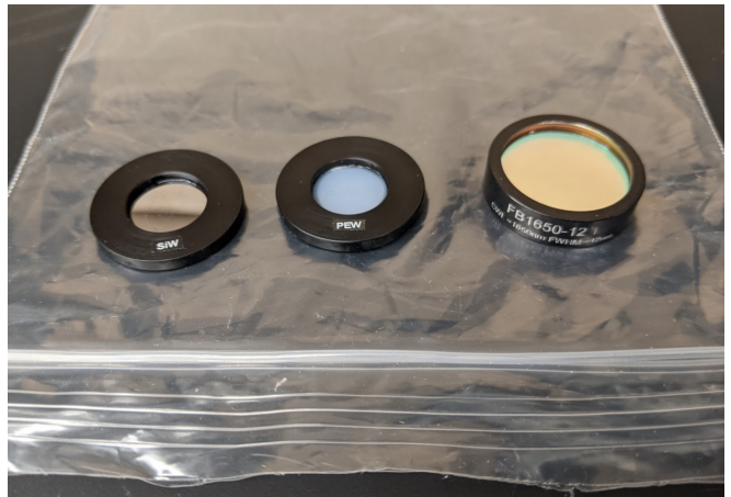
FIG. 2. Photograph of optical filters left to right: Gentec SiW (gray), Gentec PEW (light blue), Thorlabs FB1650-12 1650 nm bandpass (gold). Each are one inch in diameter, which are directly insert into the detector port. These rest on the polyethylene-based plastic bag, which is also considered as a test filter.
