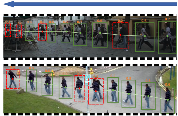
Figure 1: Illustration of tracklets generated from CStrack on two clips. Wherein, “fake background” is represented by red box. The blue arrow indicates the motion direction of the target. Best viewed in color and zoom in.
