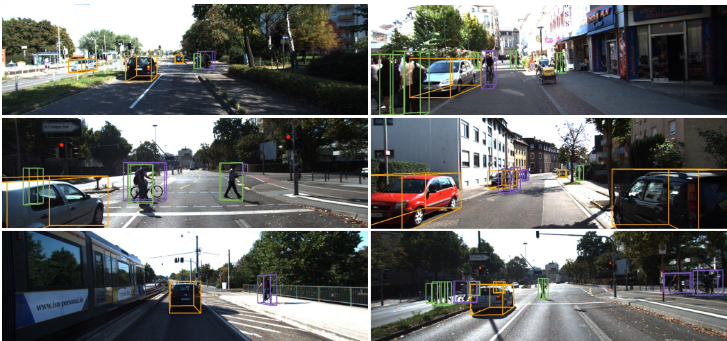
Figure 7: Qualitative results for multi-class 3D object detection. The boxes' color of cars, pedestrian, and cyclist are in orange, green, and purple, respectively.
