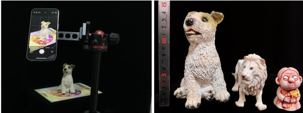
Figure 5. Our real-world data capture setup. The target object is placed on a turntable before a black background. We use an iPhone to take raw images and manually move a video light to illuminate the object from the camera side. Objects are 6 cm to 15 cm high.
