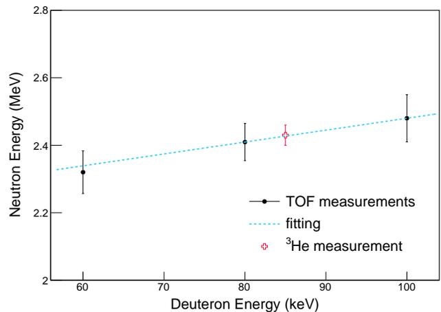
FIG. 3. The measured neutron energies from the TOF measurements as a function of deuteron energy (black dots) are shown together with  $^3\text{He}$  detector measurement (red cross) from Ref. [28]. The empirically chosen linear fit to the data is represented by a blue dashed line.
