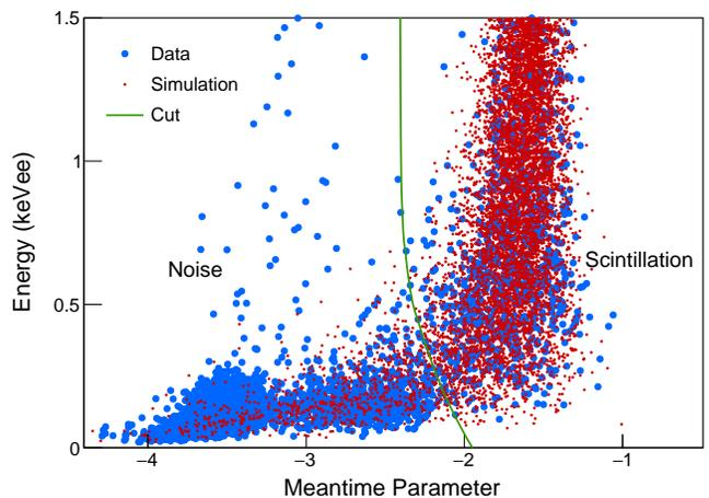
FIG. 6. Distributions of the meantime parameter for the measured data (blue points), which had a selection for the neutron scattering events, and the waveform simulation data (red points) are presented. The green-solid line indicates criteria for event selection to remove the PMT-induced noise events.
