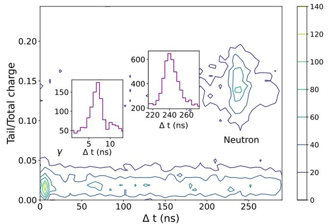
FIG. 2. The TOF ( $\Delta t$ ) of the scattered neutron in two LS detectors as a function of the PSD parameter, the tail-to-total charge ratio. Neutron and  $\gamma$  events are well separated with the PSD parameter as well as TOF. One-dimensional distribution of TOF ( $\Delta t$ ) for each particle is placed in the insets.
