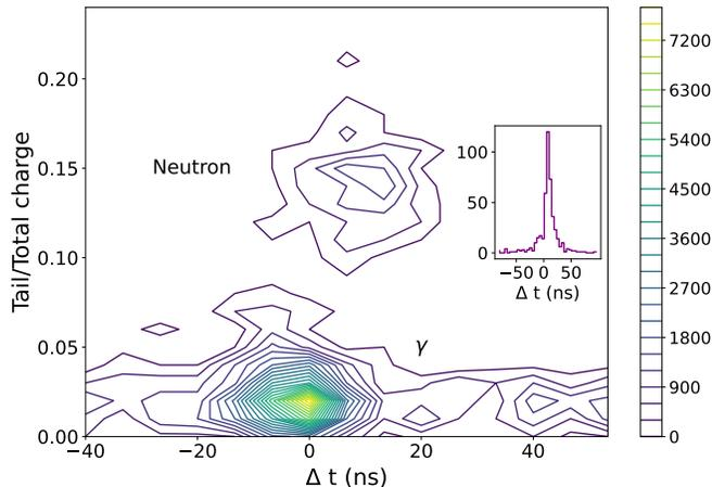
FIG. 5. The tail to total charge ratio of the LS neutron tagging detectors plotted against the TOF ( $\Delta t$ ) between the NaI(Tl) and the LS neutron detectors. Nuclear recoil events, characterized by a longer decay time in the LS detector, exhibit higher values of the tail to total charge ratio. The inset illustrates the one-dimensional TOF for the neutron event, highlighting the clear coincident timing between NaI(Tl) and neutron tagging detectors.
