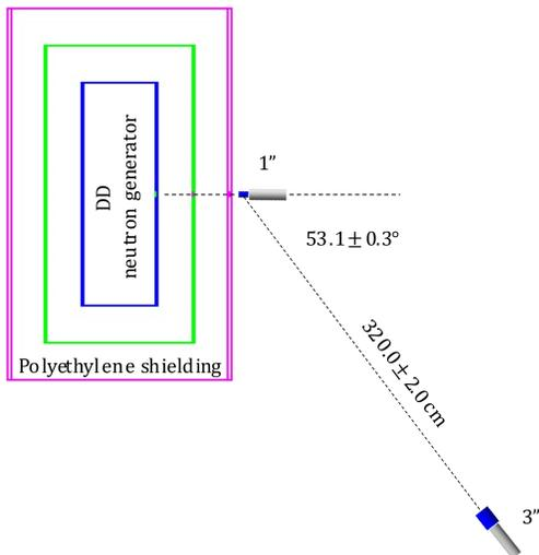
FIG. 1. Experimental setup of the incident neutron energy measurements using the TOF method. Neutrons are coming out from the deuteron-based generator inside the polyethylene shielding. One-inch diameter LS detector (LS1) is placed in front of the neutron beam direction and a three-inch diameter LS detector (LS2) is placed far from the one-inch detector to measure the TOF of the scattered neutrons.
