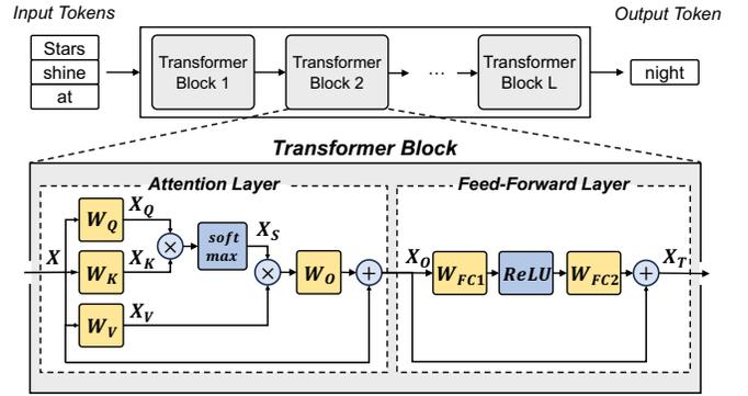
Figure 1: Illustration of the Transformer block architecture.
