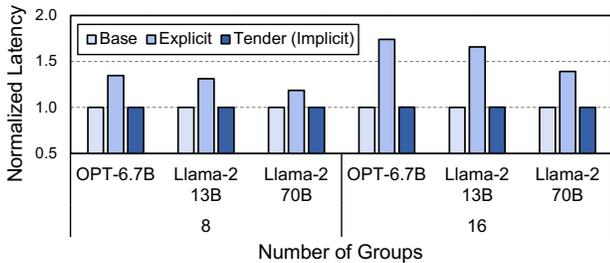
Figure 13: Comparison between implicit and explicit requantization.
