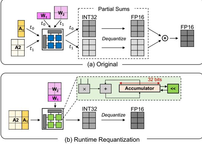
Figure 5: Runtime Requantization. Compared to the original computation flow, we retain the reduction axis length by shifting the accumulated partial product sum between decomposed matrices.
