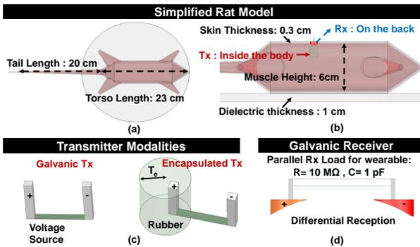
Fig. 3. (a) Top view and (b) side view of the simplified rat model, showing the implementation of Tx and Rx. (c) Pure galvanic Tx and encapsulated Tx to mimic the capacitive implant Tx. (d) The Galvanic Rx model.
