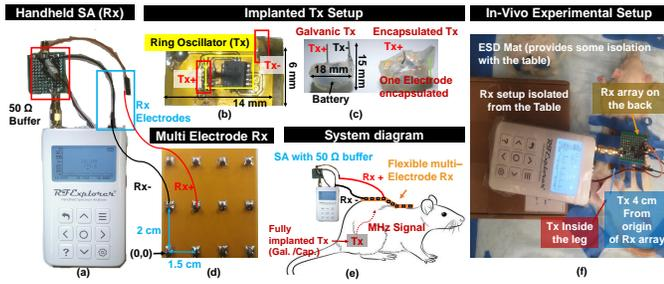
Fig. 5. (a) RF Explorer handheld spectrum analyzer (SA) with  $50\ \Omega$  buffer, connecting to a multi-electrode Rx. (b) The Flexible Tx Implant, featuring a battery-powered ring oscillator. (c) Side view of the set up, showing galvanic Tx and encapsulated Tx. (d) Multi electrode array taped on the rat's back to measure Rx signal. (e) Full system diagram. (f) In-vivo measurement setup.
