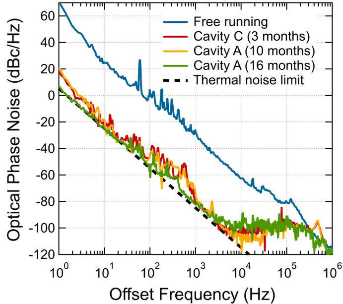
**Fig. S1.** Phase noise measurements on a 1550 nm laser stabilized to other in-vacuum bonded cavities, referred to as Cavity A and C, at different times after the cavities were bonded. Also shown is the free running laser noise and the cavities’ estimated thermal noise limit. The 16-month measurement was performed in a different system with more optimized settings compared to that of the other two measurements.
