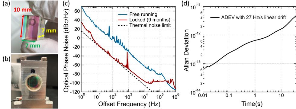
Fig. 5. Measurements on the in-vacuum bonded cavity with lithographically fabricated mirror. (a) Photograph of the cavity under test that was diced out of an array of cavities. (b) Photograph of the cavity inside the air-tight metal enclosure. (c) Phase noise measurement on a 1550 nm laser stabilized to the cavity. Blue: free running laser noise. Red: phase noise at 9 months after bonding. Black: estimated thermal noise limit of the cavity. (d) The corresponding measured Allan deviation.
